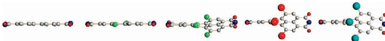
Figure 5. Side view onto the aromatic systems of 1a–e (from left to right) showing a progressive twist of the perylene core. The angles are 1.5° for 1a , 3.0° for 1b , 19°/26° for 1c , 35°/36° for 1d , and 37° for 1e .
